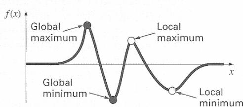
A function that asymptotically approaches zero at plus and minus  $\infty$  and has two maximum and two minimum points in the vicinity of the origin. The two points to the right are local optima, whereas the two to the left are global.
